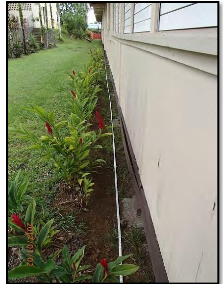
Soil contaminants from historic practices (e.g. use of lead paint or pesticides) can be suspect in building perimeter areas.
