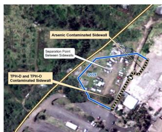
Example of map noting specific areas of residual contamination onsite as well as types of contamination.
