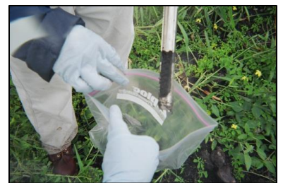
Top – Collection of soil sample with soil core sampler equipped with a T-Handle. Bottom – Soil increment deposited into labeled Ziploc bag.
