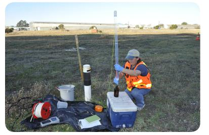
Monitoring natural attenuation at the site by collecting a groundwater sample.
