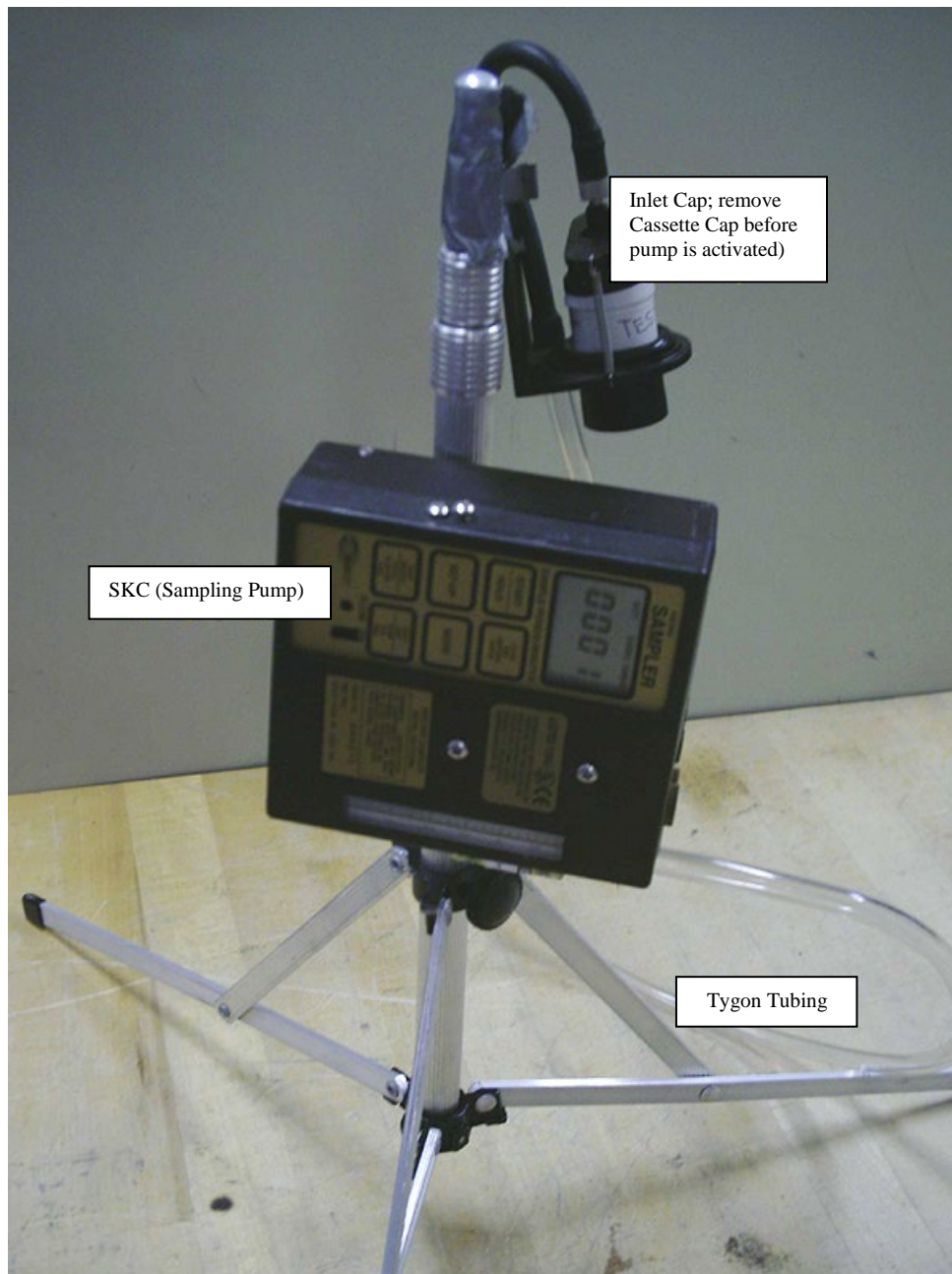
FIGURE 5. Personal Sampling Train for Asbestos
