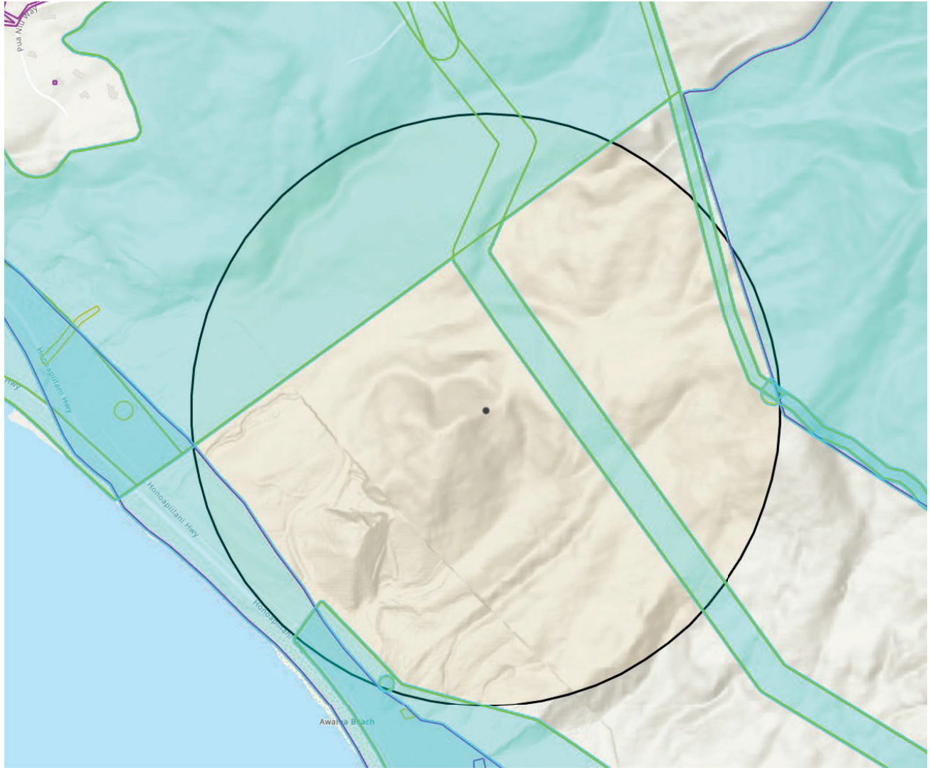
Figure 5. Figure shows 0.5-mile buffer that serves as Indirect APE for capture viewshed for Site 1TDSR. Site 1 is represented by black dot in the center of the circle.
