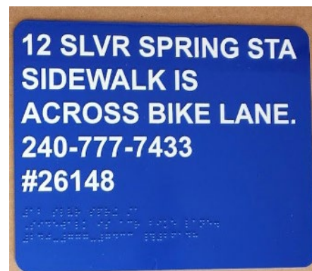
Figure 54: Example of tactile raised letter sign with bus information
