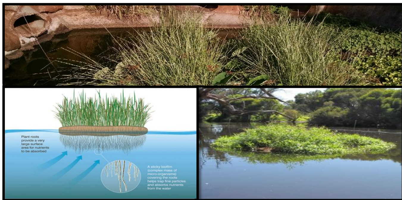
Figure 42. Floating Treatment Wetland Examples
