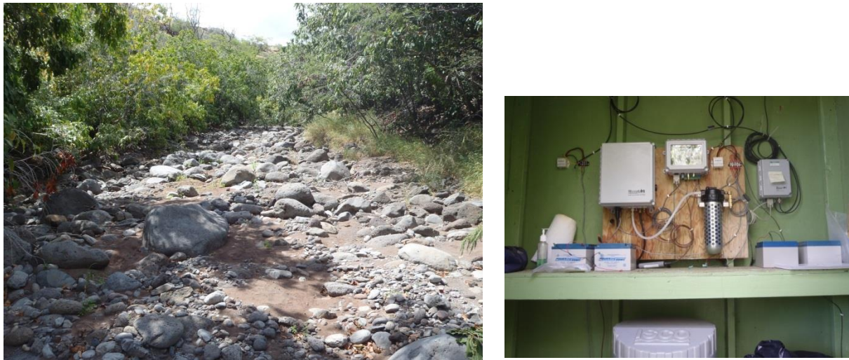
Figure 5. Kawela stream gauge with ISCO automated water sampler and pressure sensor.
