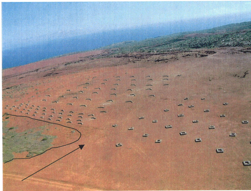
Figure 48. Combination of 91 “C-Shapes” and “Planter Boxes” in Tier I (surface cleared only) downwind of a native planting area on Kaho’olawe.
