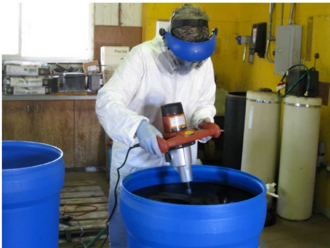
Figure 4-5: Mixing fluorescein in 55 gal. drums.
