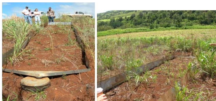
Left-surface runoff was collected to determine which groundcover (oats, sun hemp or sudex) was most effective to reduce soil erosion and nutrient loads; Right- View down slope of the test plot segregated from the field with galvanized divisions.
