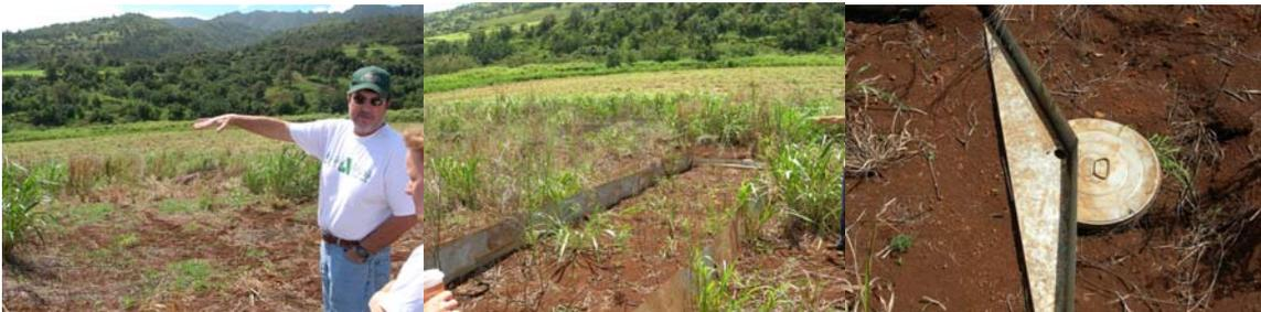
*Photos of a test plot and water collection device in the Kaiaka-Waiialua Watershed; surface runoff is monitored for sediment and nutrients from four different demonstration crop cover plots*
