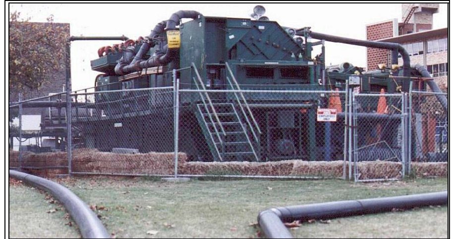
Figure 21. Sediment from Water Separator. The Separator is mounted on two semi-trailers, part of a Lake Merritt dredge system. One pipe brings dredged sediments, a liquid material, to the Separator and the second pipe returns water (sediments removed) to the Lake. The Separator discharges the sediment removed from the water directly to a dump truck for transport to a landfill.
