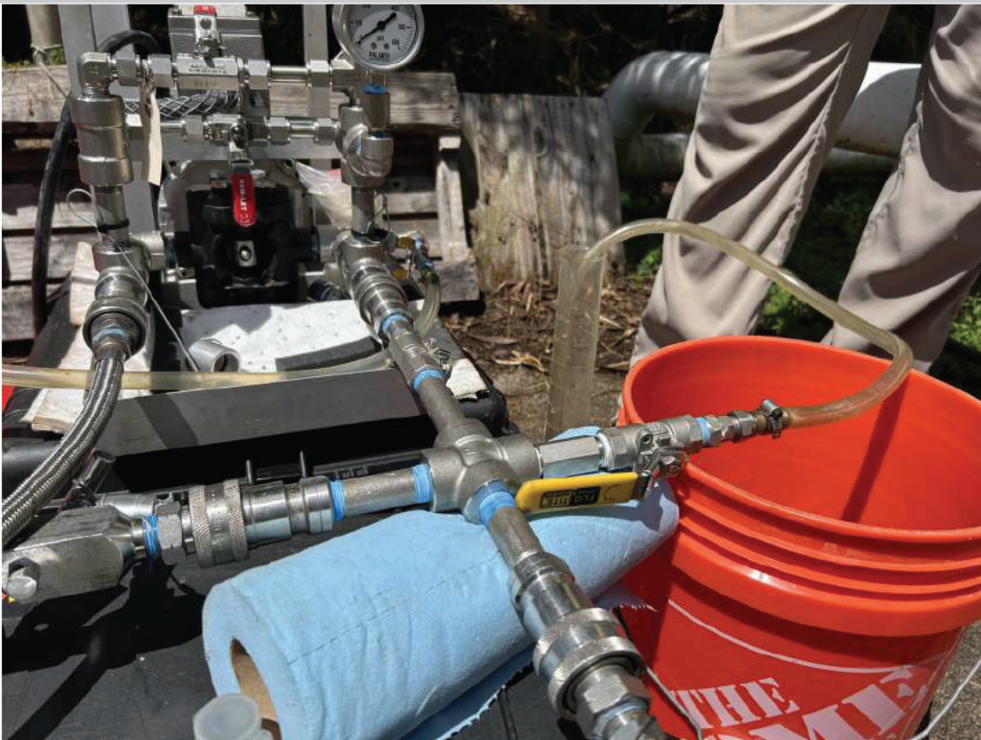
Simulated leak testing performed as part of leak detection testing.
