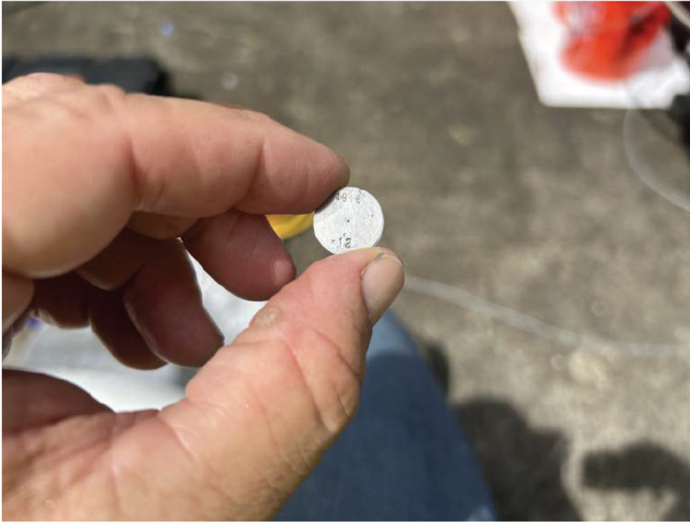
Orifice plate utilized for simulated leak testing.
