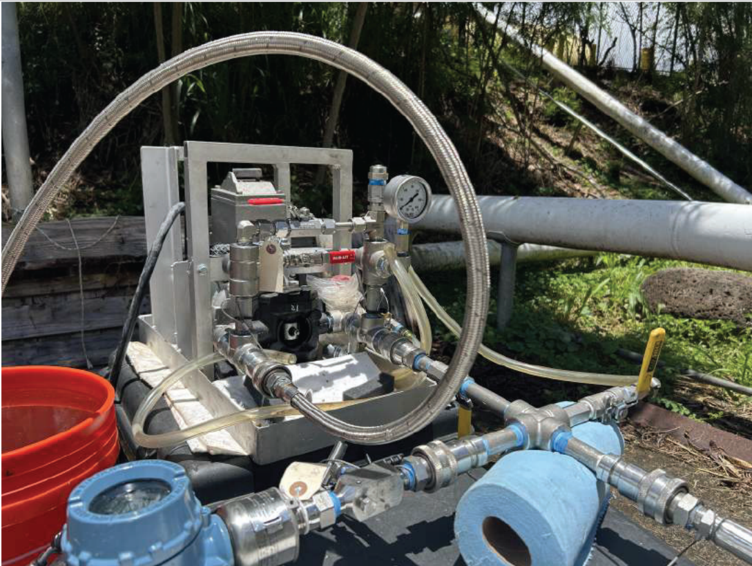
Pump and test tree assembly outside Tank S311 for pressure step leak detection testing.
