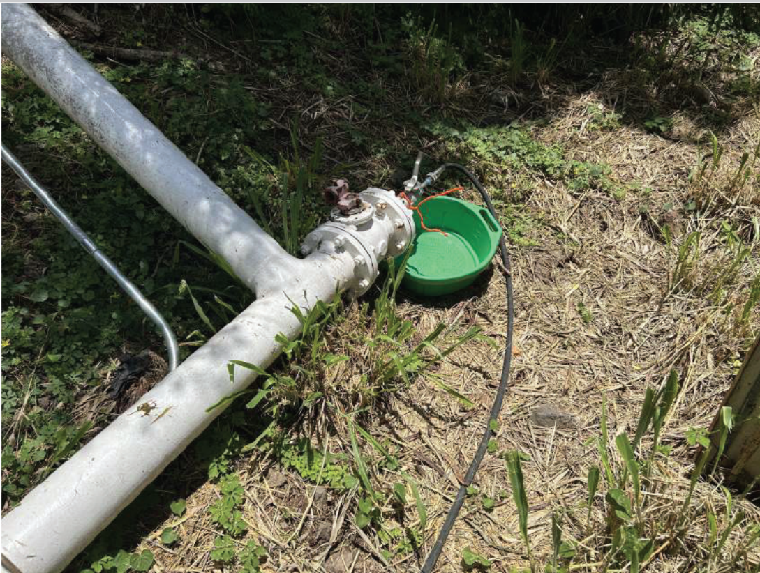
Containment staged at each hose connection for leak detection testing.
