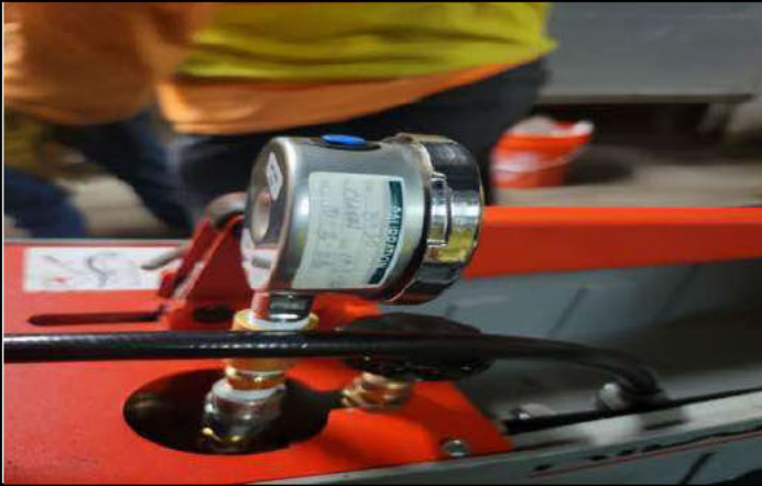
Calibrated 0-300 pressure gauge.
