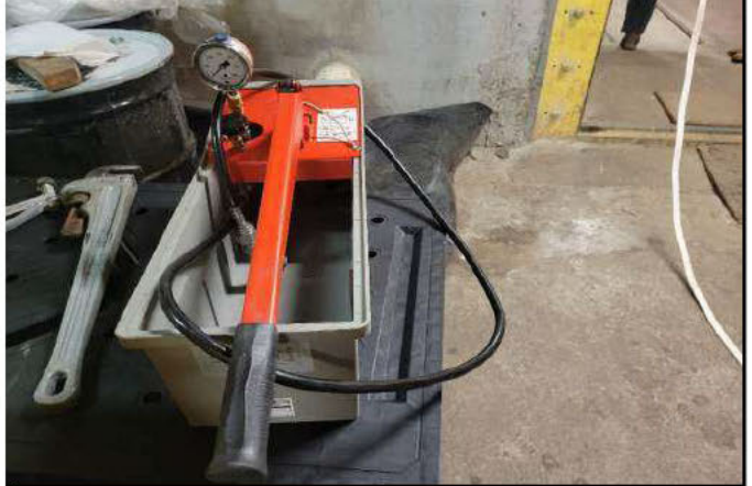
Hydrostatic pressure testing pump.
