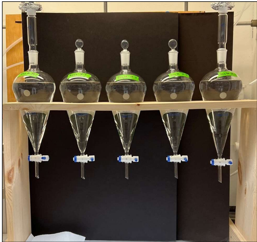
Figure 1. Photographs of water-fuel experiments: A) Experiment setup using one-liter funnel flasks (L-R: Day 0, Day 5, Day 10, Day 15, Day 20); B) Closeup of 10 ml layer of JP-5 fuel placed on top of one liter of water.
