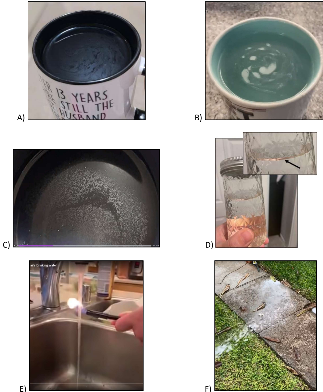
Figure 1. Sheens and gel-like emulsions and foams in tapwater from residences following release of JP-5 jet fuel into JBPHH drinking water system (Hawaii News Now 2021a). A) Fuel sheen on tapwater from JBPHH resident home (Hawaii News Now 2021a,b); B) Foamy residue on tapwater from JBPHH resident home (Hawaii News Now 2021b) C) Emulsion-like material on tapwater from JBPHH resident (HNN 2021c); D) Approximately one-millimeter thick layer of gel-like emulsion on sample of fuel-contaminated; tapwater collected by JBPHH resident (used with permission from resident); E) Flammable vapors from fuel-contaminated tapwater at a JBPHH residence (Vice News 2022); F) Foamy residue from garden hose of JBPHH resident home (used with permission from resident).
