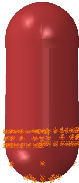
Figure 5-19 – Boundary Conditions in the Model, Tank Elevation
