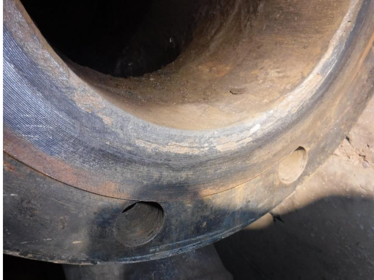
C.37 Crevice corrosion flange gasket face 0.030" to 0.040" deep (entry point B)
