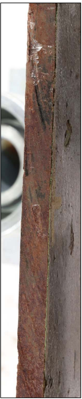
Figure 9. An image of a representative edge of Coupon 3 in the as-received condition.
