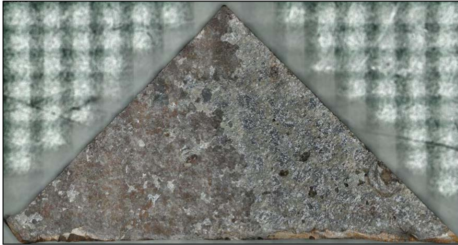
Figure 169. A screenshot of the 3D digital image of a specimen excised from Coupon 8 labeled as 8-2, after CO 2 blast cleaning
