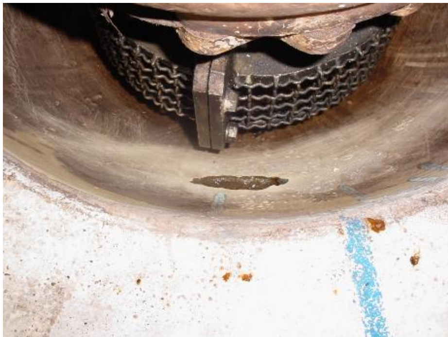
Wear Hole in Sump
