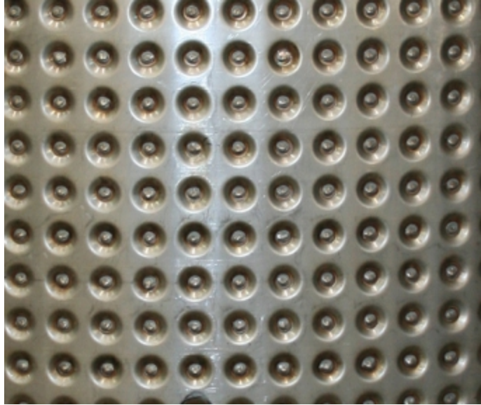
Closeup of Dimples in Jacket
