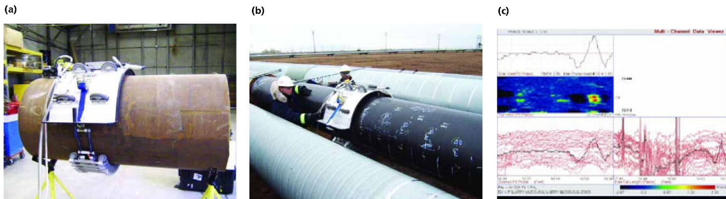
Figure 8. LFET axial scanning array; (a) closeup in trial configuration, (b) in use on petroleum transit pipeline, and (c) LFET data from pipe segment in trial configuration in 8a (compare to C-scan image of pitting in same pipe segment in Fig. 7c).
