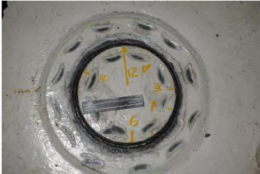
Photo 7: Tank Drain Line Cap (Note: Indications found with Magnetic Particle Testing).
