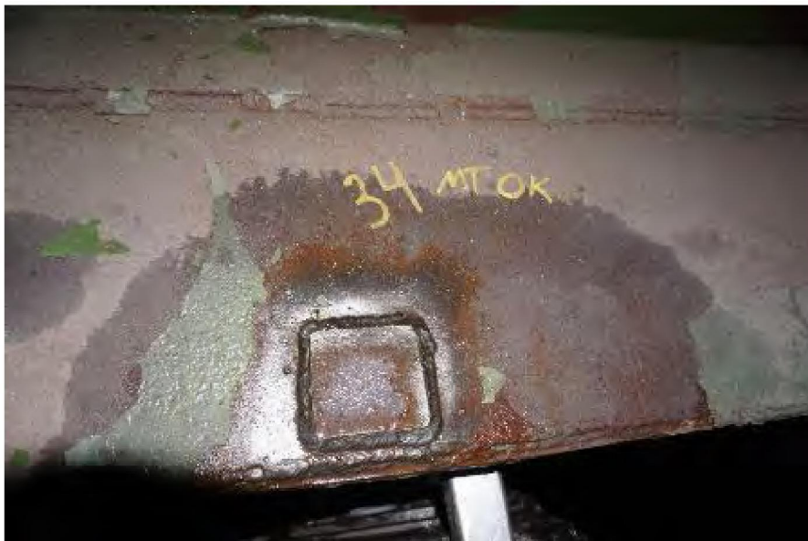
Photo 26: Extension Ring Plug Welds
