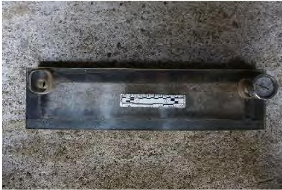
Photo 39: Vacuum Box EEI-001 for linear weld testing
