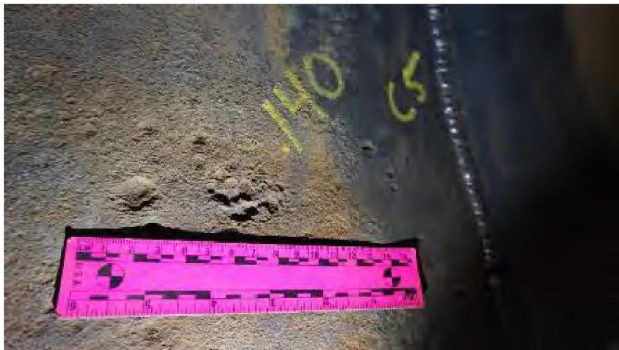
Photo 16: 32-inch piping interior pitting
