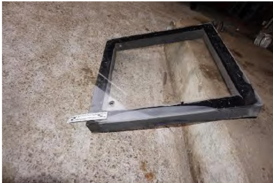
Photo 40: Vacuum Box EEI-006 for small Patch Plate weld testing
