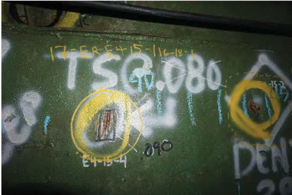
Photo 16: Gouge in extension ring plate
