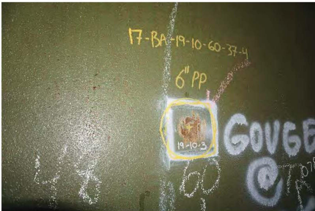
Photo 19: Gouge on barrel plate
