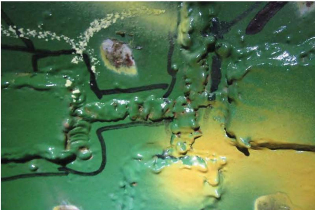
Photo 12: Poor welds between the backing bars of four plates on upper dome
