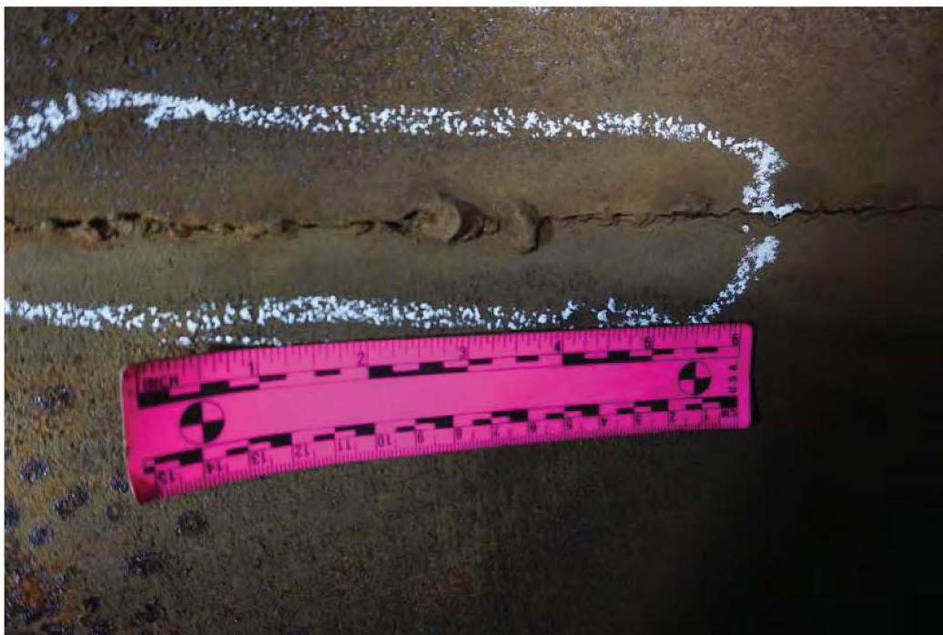
Photo 19: Weld defects of circumferential weld in 32-inch piping.
