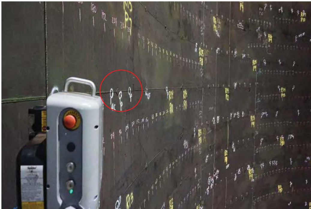
Photo 10: Inspection marks (chalk, white and yellow paint) on liner plates in the barrel. Area circled in red shows example of relevant indications of weld discontinuities.
