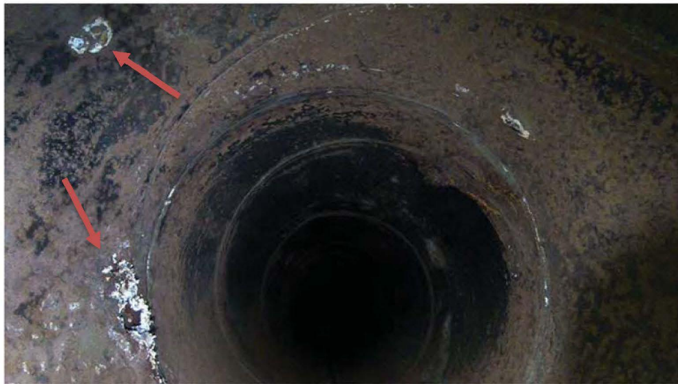
Photo 3: Corrosion resulting in hole along welds with possible calcium deposits.
