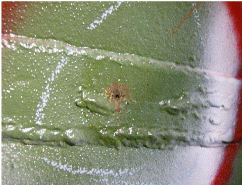
Flaw 347 through hole in strap
