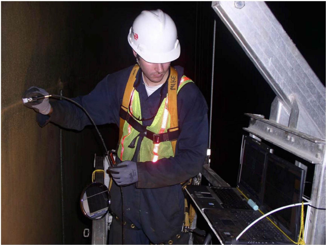
Above: The Hawkeye Pencil Probe used for testing all welds in tank # 2. Below: A TesTex crewmember using the Hawkeye a weld from one of the baskets.
