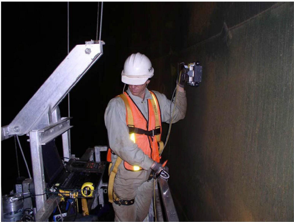
Above: A specially developed 8” wide hand scanner used for the majority of the surface scanning. Below: A TesTex crewmember using the hand scanner from one of the baskets.
