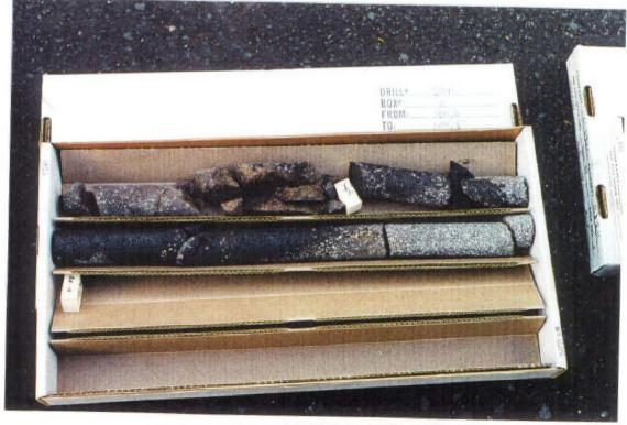
Figure 4-10 Petroleum Stained Core - B16A, 100' to 104'
