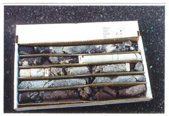
Figure 4-9 Petroleum Stained Core - B16A, 81' to 91'
