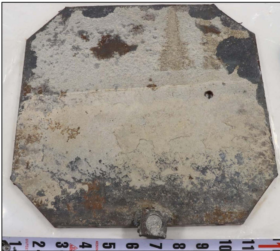
Figure 10. An image of the interior surface of Coupon 5 in the as-received condition.
