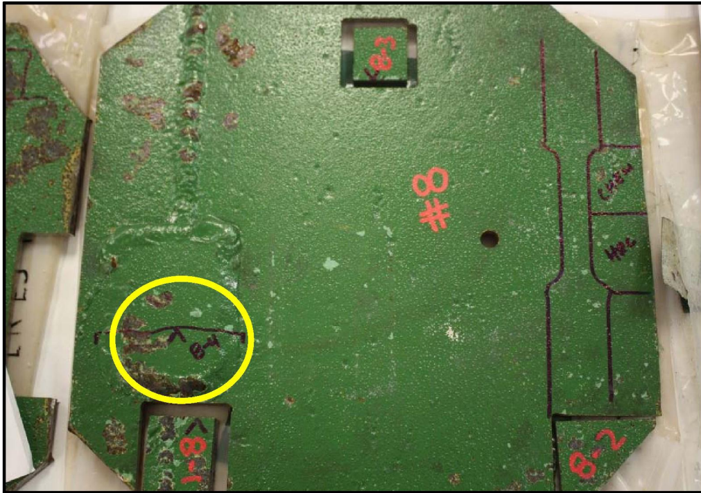
Figure B-5. Coupon #8 photograph showing the location of metallographic specimen 8-4 in relation to 8-1, 8-2 and 8-3.
