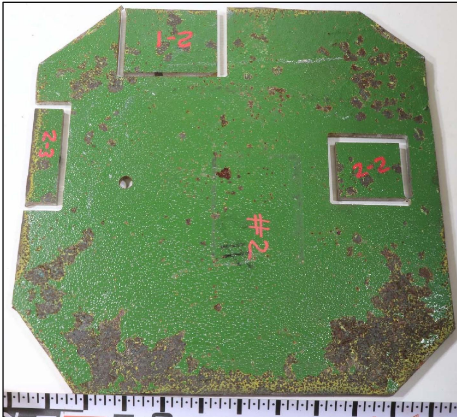
Figure 132. An image of the exterior surface of Coupon 2 after CO 2 blast cleaning.
