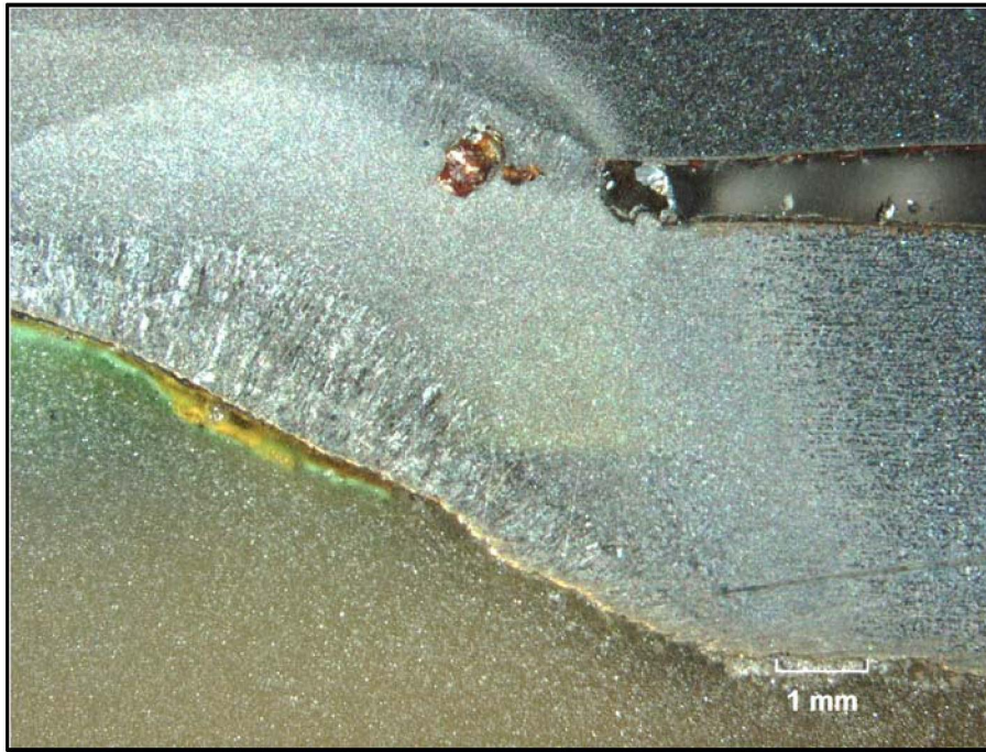
Figure 211. The left-hand feature in Figure 210 is shown at higher magnification. The weld indication (arrow) appeared to be an area of porosity.
