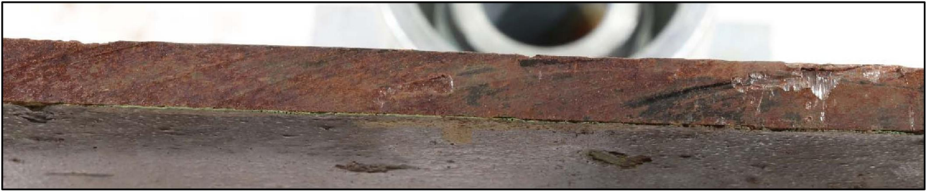
Figure 9. An image of a representative edge of Coupon 3 in the as-received condition.
