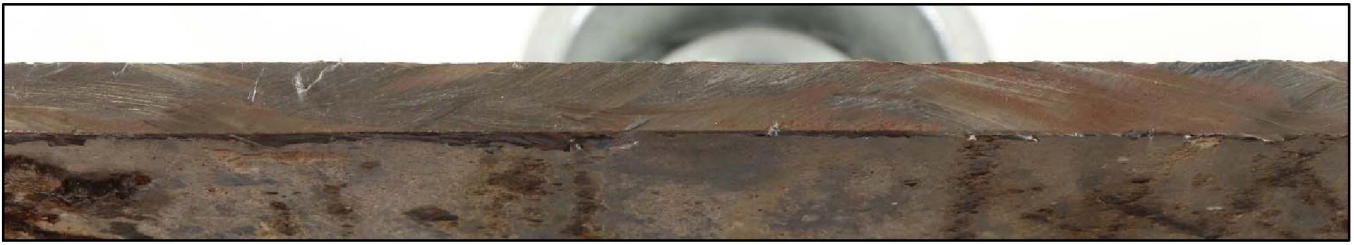
Figure 3. An image of a representative edge of Coupon 1 in the as-received condition.
