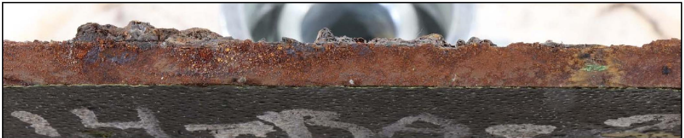
Figure 18. An image of a representative edge of Coupon 7 in the as-received condition.
