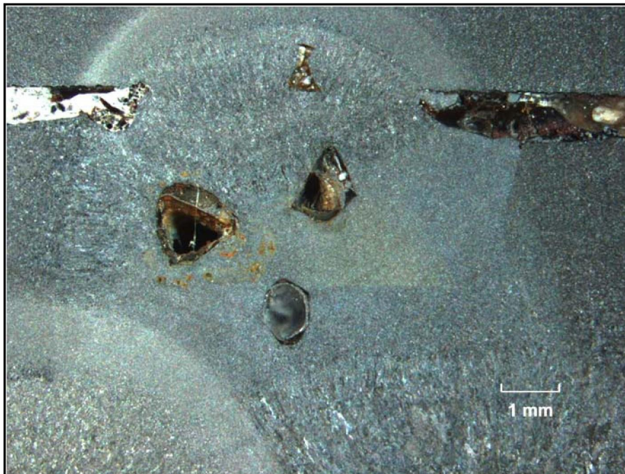
Figure 212. The right-hand feature in Figure 210 is shown at higher magnification. The weld indications appeared to be porosity.
