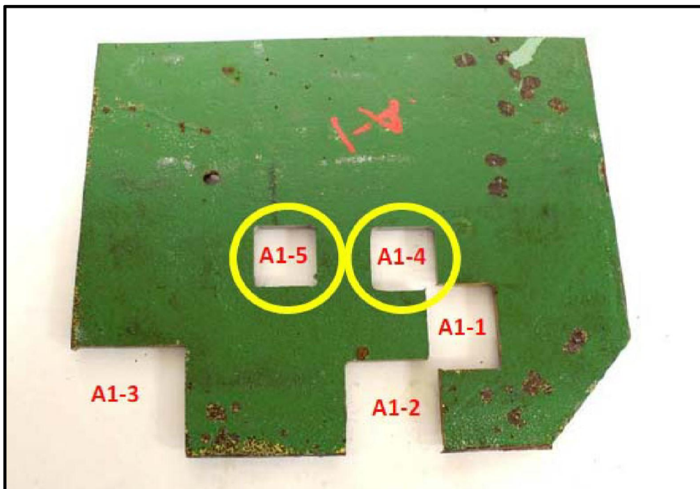
Figure B-6. Coupon #A1 photograph showing the location of metallographic specimens A1-4 and A1-5 in relation to A1-1, A1-2 and A1-3.
