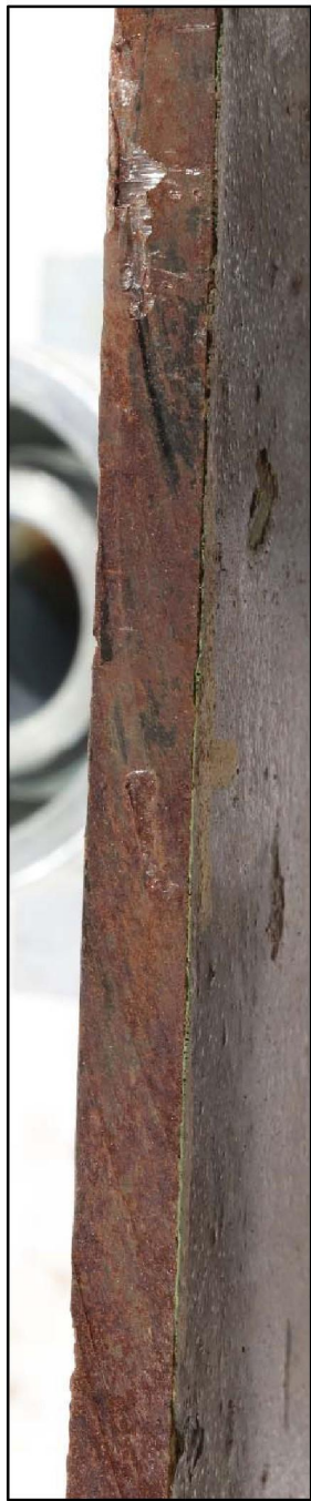
Figure 9. An image of a representative edge of Coupon 3 in the as-received condition.
