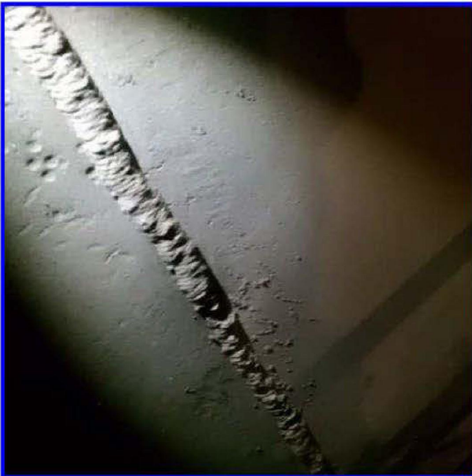
Length of weld with moderate to extensive weld spatter IR-1
