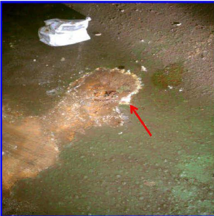
Visible salt on flat bottom of tank IR-1
