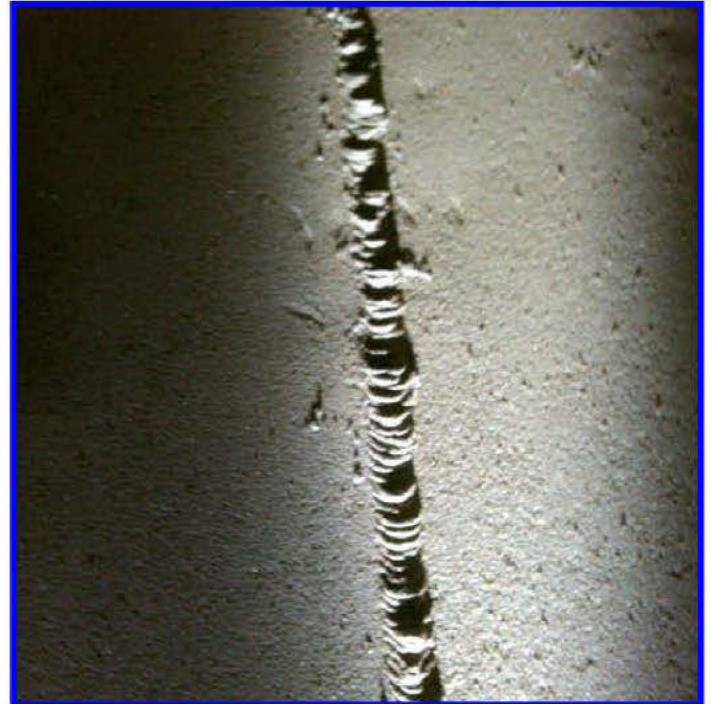
Length of weld with less extensive weld spatter
