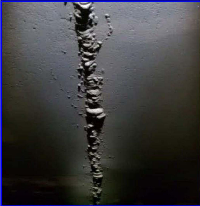
Length of weld with extensive weld spatter
