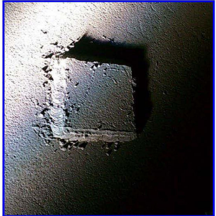
4\"X4\" welded plate with extensive weld spatter
