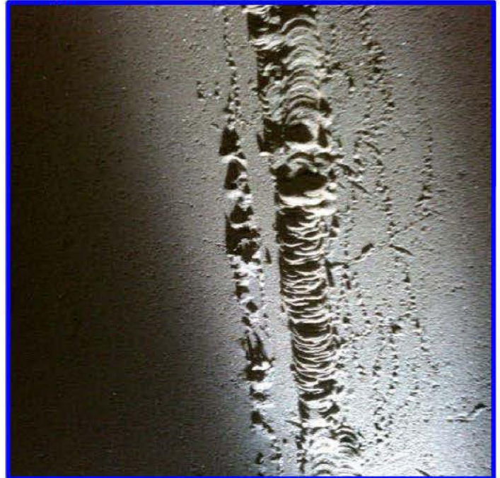
Length of weld with extensive weld spatter
