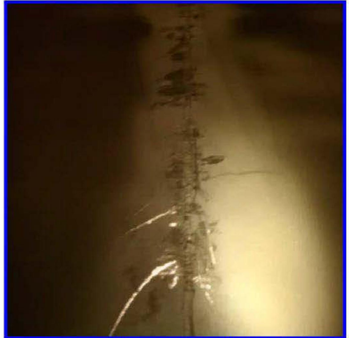
Length of weld with less extensive weld spatter that had been grinded
