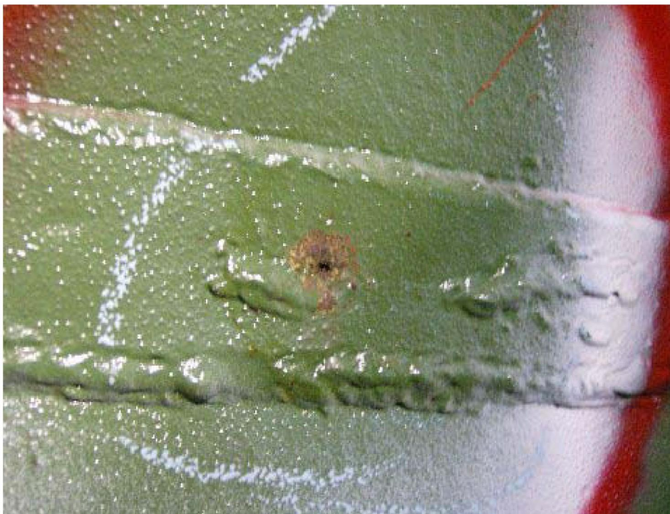
Flaw 347 through hole in strap
