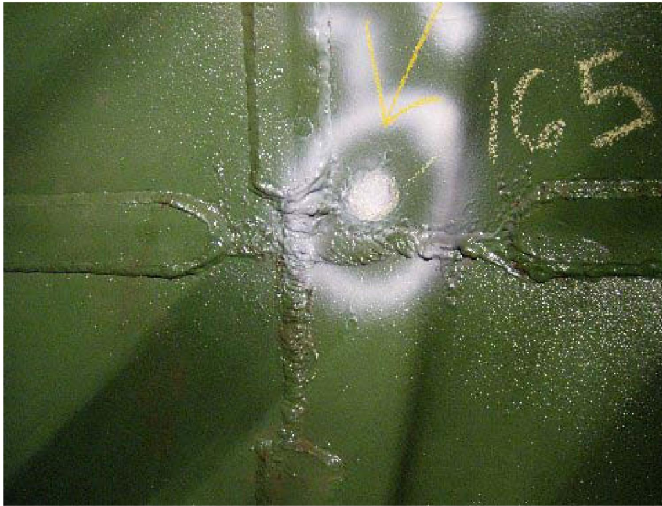
Flaw 304 Loss of Wall measured .165"
