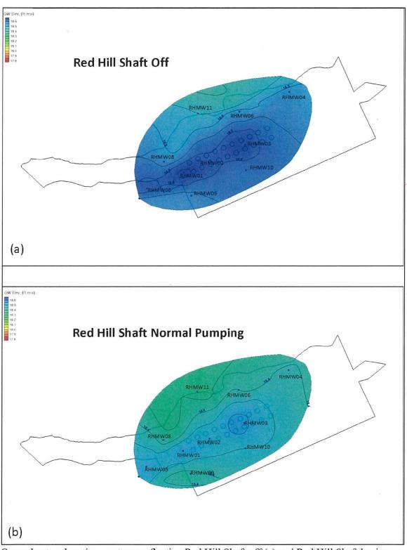
Groundwater elevation contours reflecting Red Hill Shaft off (a) and Red Hill Shaft business as usual (b) pumping conditions as reported by the Navy<sup>10</sup>.
