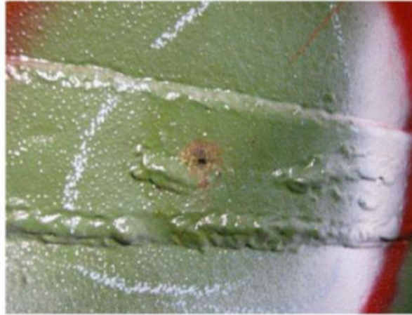
Flaw 347 through hole in strap
