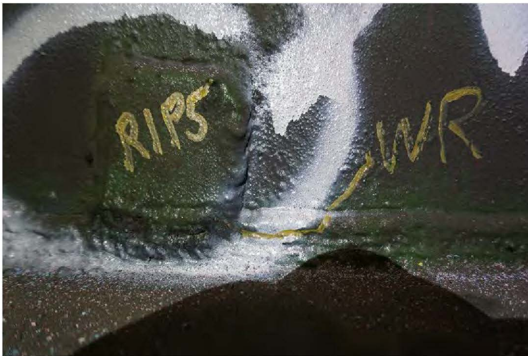
Photo 12: Example of a relevant indication in previous patch plate welds on barrel plate in row 1.
