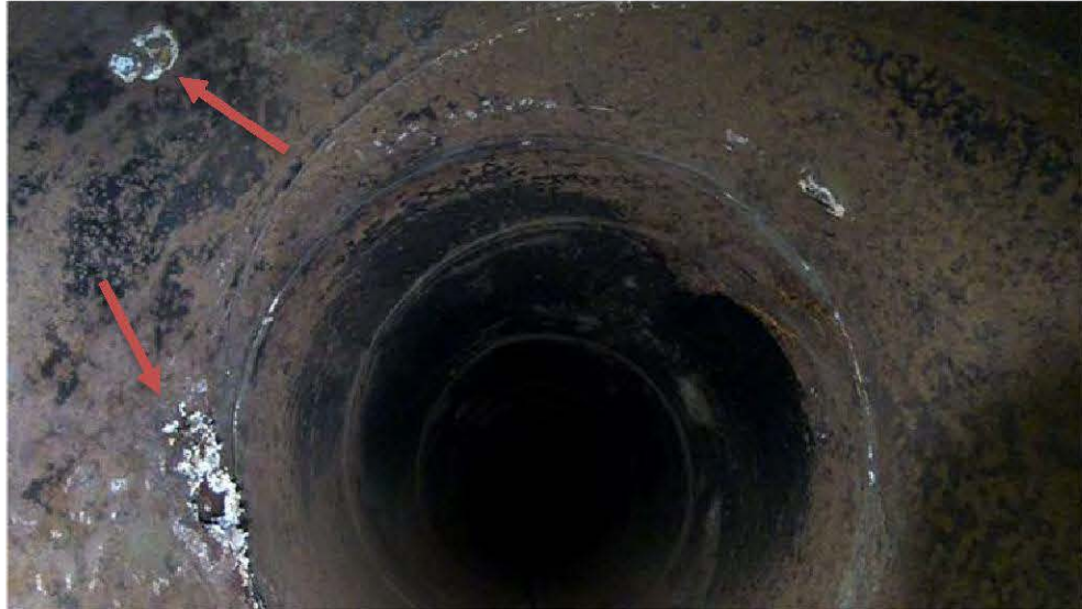
Photo 3: Corrosion resulting in hole along welds with possible calcium deposits.
