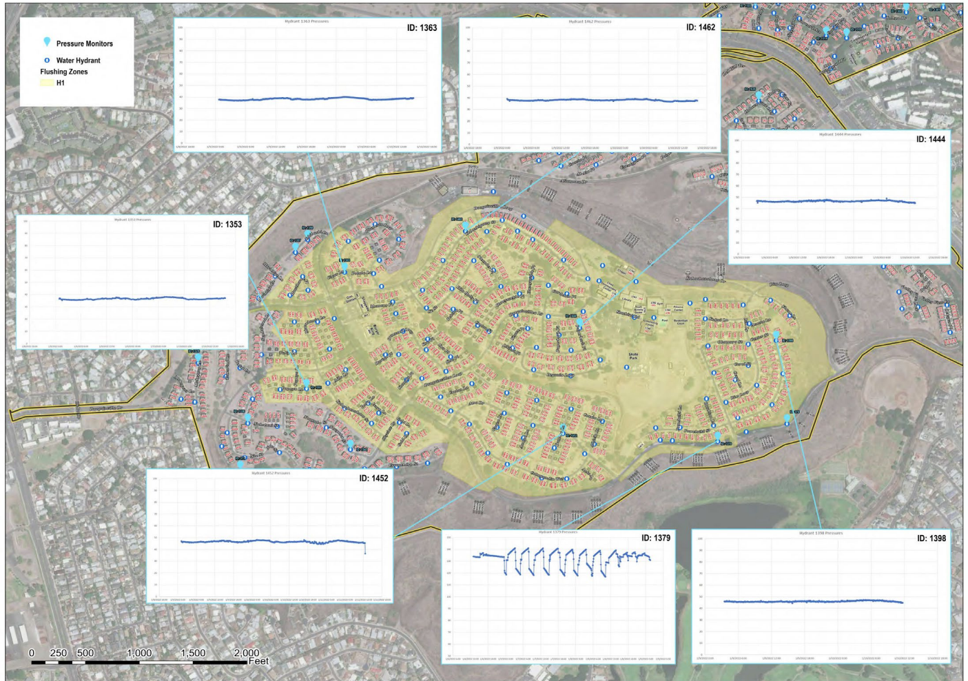
FIGURE 1: DISTRIBUTION FLUSHING PRESSURE DATA (January 2022) Zone H1
