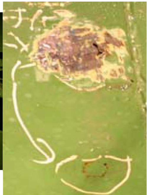
Figure 5. Photographs extracted from the API Tank 16 Inspection Report (Photograph 8) showing "holes at the top of course F of the upper dome".
