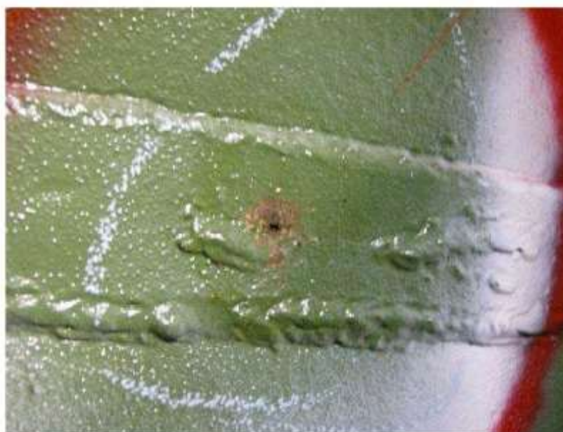
Flaw 347 through hole in strap
