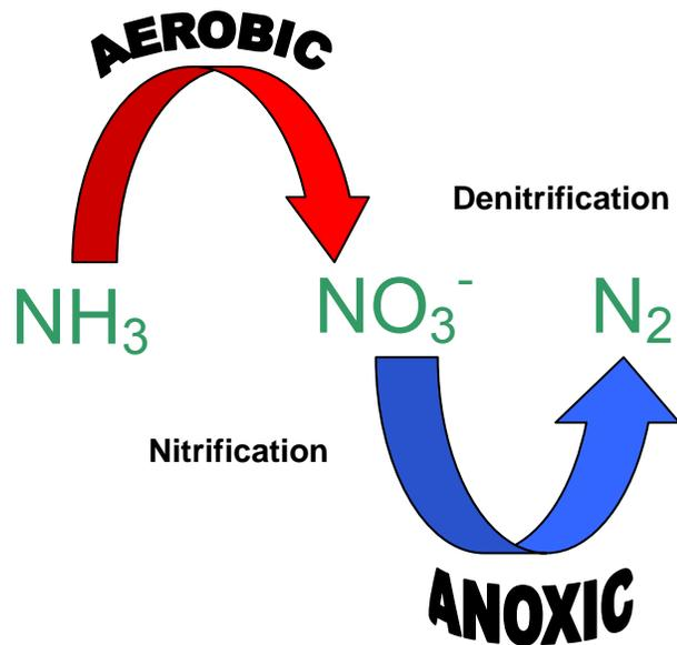
**Figure 5-7 The Removal of Nitrogen from Wastewater**
