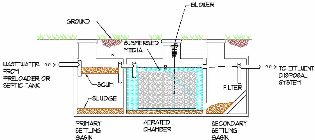
**Figure 5-4 Combined Attached and Suspended Growth Reactor**
