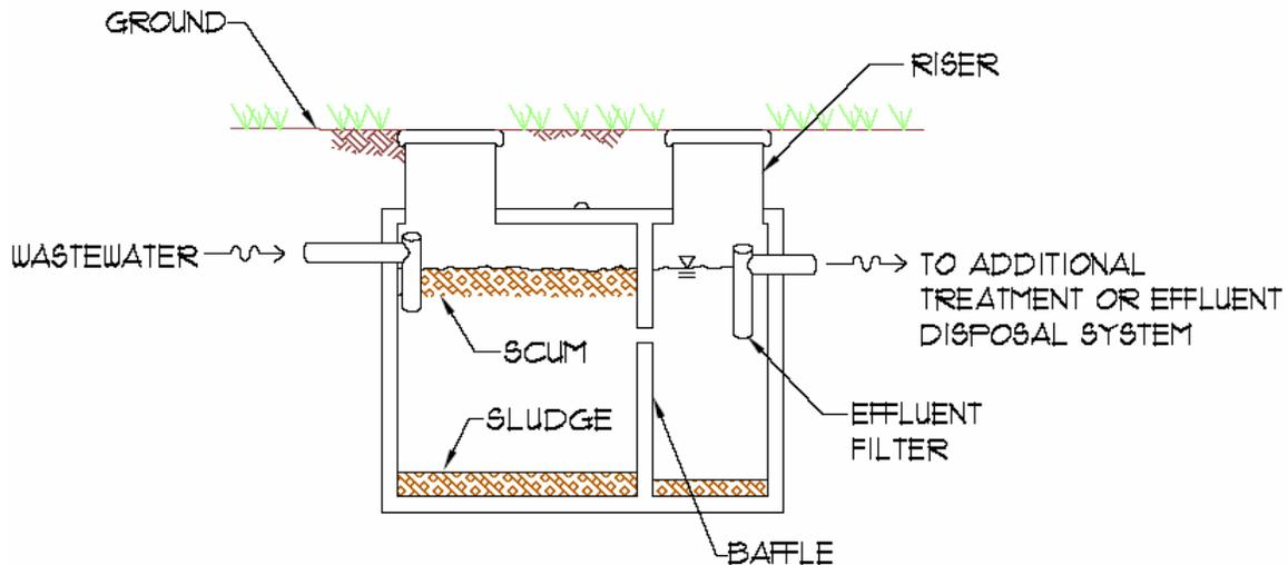
**Figure 5-2 Typical Double Chambered Septic Tank**
