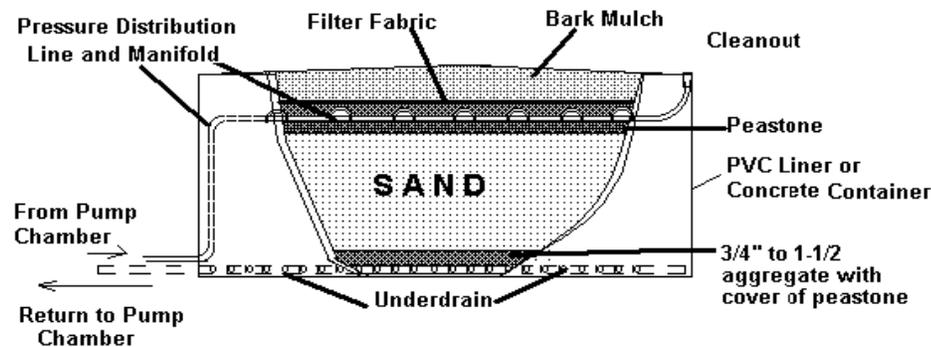
**Figure 5-6 Packed Bed Filter (Adapted from USEPA)**
