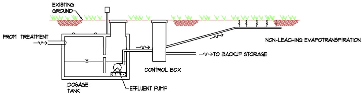
**Figure 4-6 Subsurface Evapotranspiration Profile of Typical ET System**
