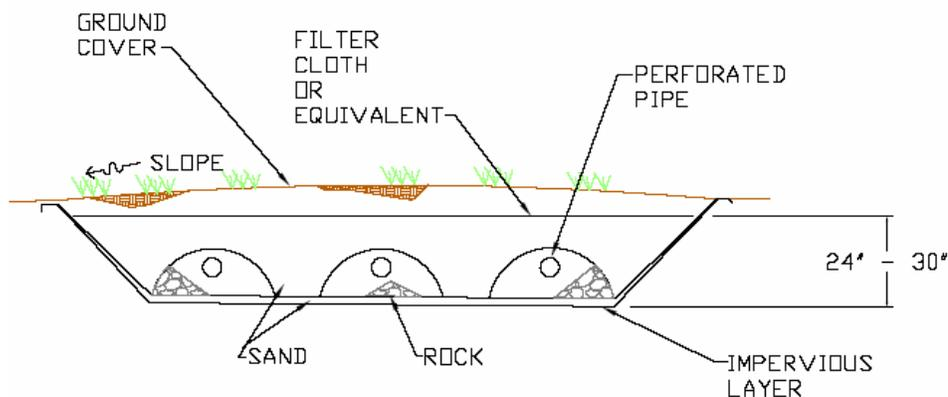
**Figure 4-5 Cross Section of an ET Bed**
