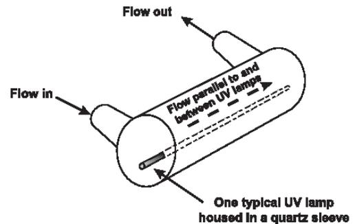
**Figure 5-9 Ultraviolet Radiation Chamber (Adapted from USEPA)**
