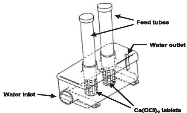
**Figure 5-8 Tablet Chlorination Chamber (Adapted from USEPA)**
