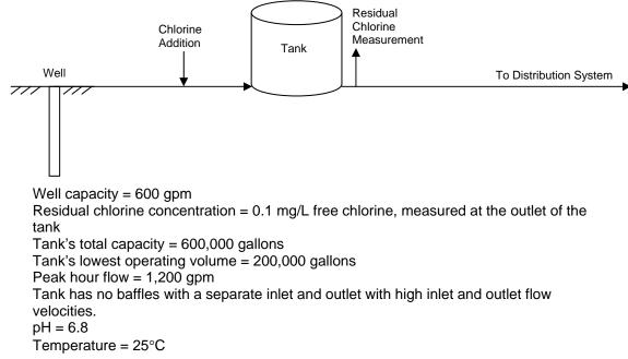
FIND If the water system is providing 4-log virus inactivation.
