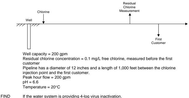
NOT RELEVANT - The well capacity has no bearing on the peak flow of the water system.
