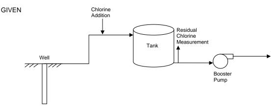
Well capacity = 100 gpm Residual chlorine concentration = 0.1 mg/L free chlorine, measured at the outlet of the tank Tank's total capacity = 50,000 gallons Tank's lowest operating volume = 25,000 gallons Booster pump capacity = 250 gpm Tank has no baffles with a separate inlet and outlet. The inlet is located at the top of the tank and the outlet is located at the bottom of the tank on the opposite wall. pH = 7.5Temperature = 20°C
